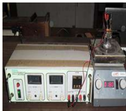
Fig 1. Electro-deposition Setup in the laboratory
