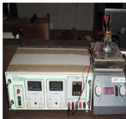
Fig 1. Electro-deposition Setup in the laboratory
